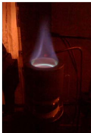
Figure 2-7: Fuel Burn Off at the Reactor Exit.
